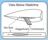
A flexible strip for sealing the centreboard or daggerboard slot on dinghies, catamarans and sailboards. It has also found use as transom flaps and as rudder fairings on cruisers.
